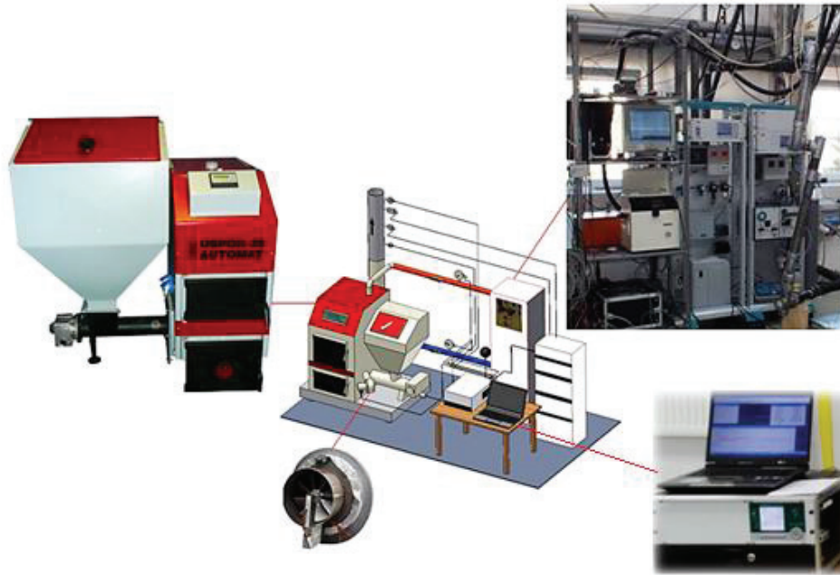
FIGURE 1. Experimental measurements boiler
