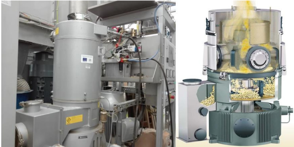
Obr. 6 Peletovacie zariadenie KAHL 33-390/500 ( www.directindustry.com )
