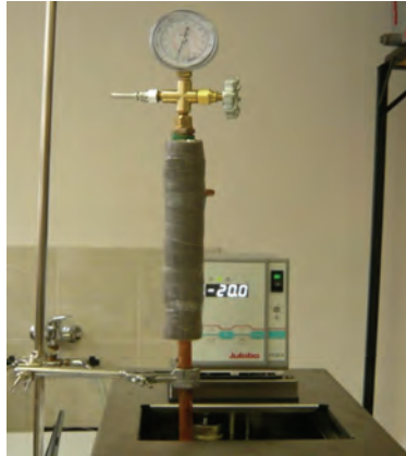
Fig. 1. Heat pipe in an ice bath to 0°C and cooling thermostat to 20°C
